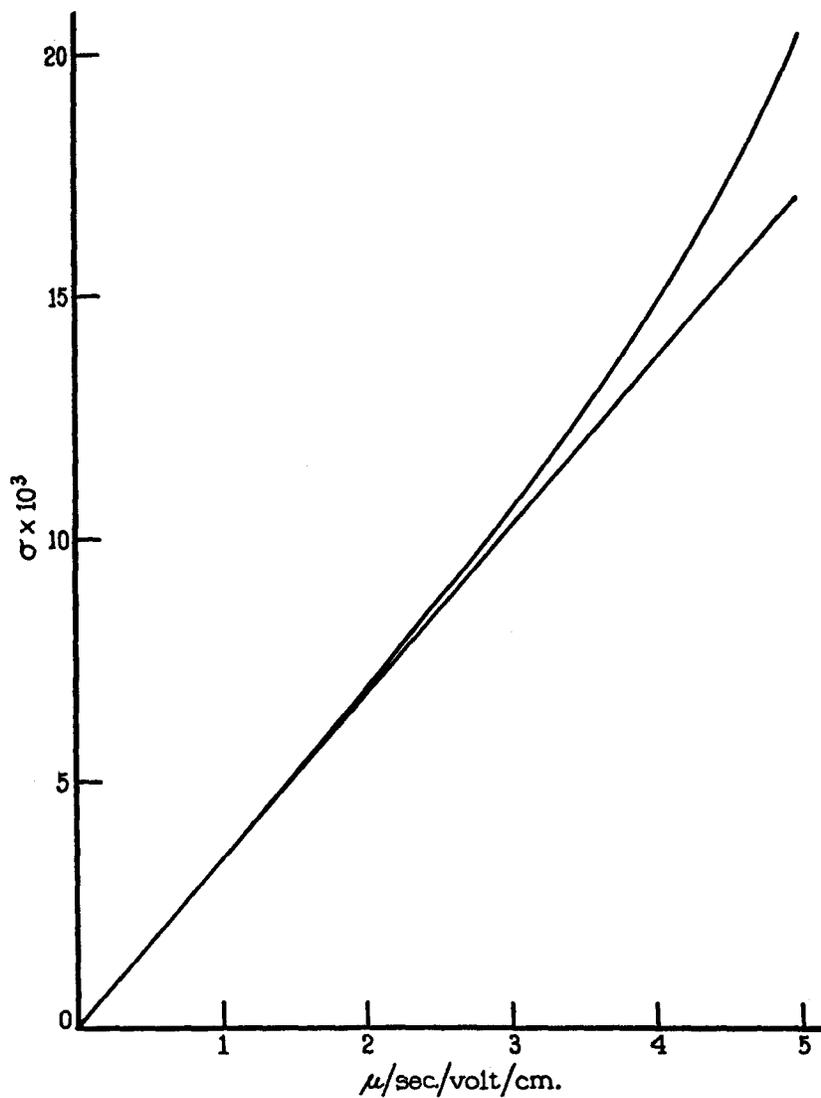
FIG. 1. The straight line has been calculated according to the Debye approximation and the curved one by means of equation (2) for  $\pi/15$  phosphate buffer.
