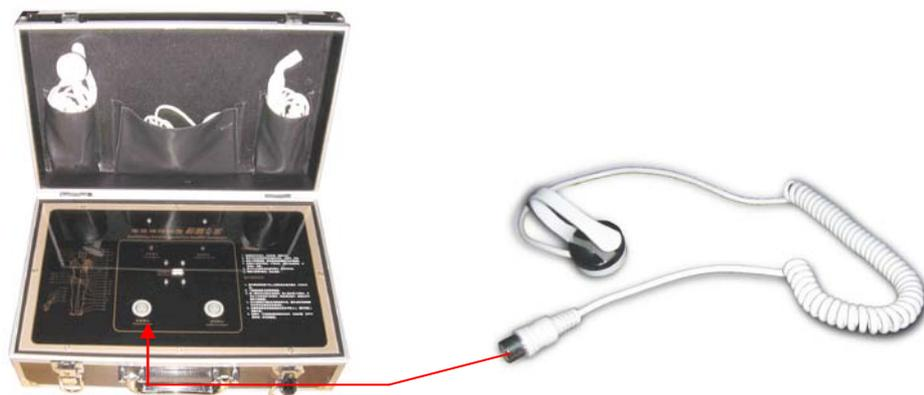
3. The square end of USB extension line is connected to USB Output in the instrument, the other flat end should be inserted to the computer's USB interface.
